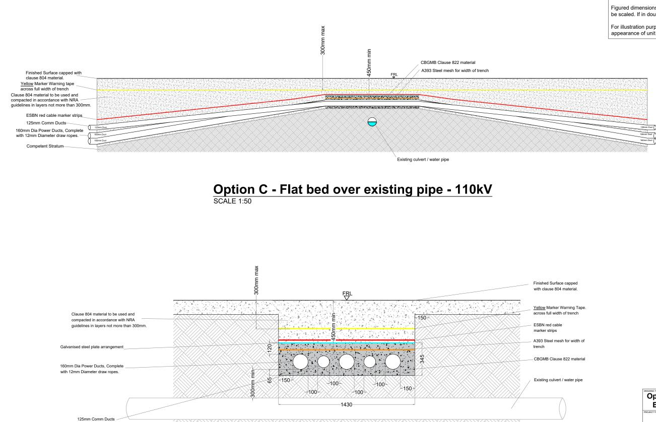
Option C - Flat bed over existing pipe - 110kV
